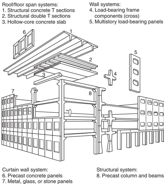
**FIGURE C.1(k) Precast Concrete Frame.**
