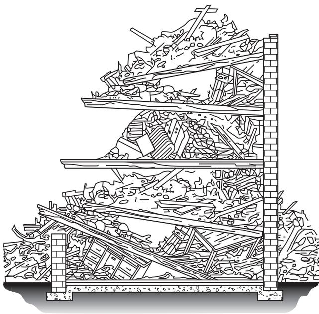
FIGURE I.1(d) Cantilever Floor Collapse. (Courtesy of U.S. Department of Civil Defense)
