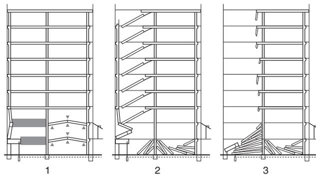
**FIGURE I.2(i) Lift and Drop Collapse Pattern — Concrete Heavy Floor Construction.**
