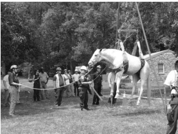
**FIGURE J.3.4** The Becker Sling System. Here it is used in a vertical lift of a live animal [weighing 1325 lb (601 kg)] with a TLAER-rated A frame. The overhead features two lifting points and an emergency release system. The breast strap does not impede the trachea — it just holds the strap behind the front legs in position. The lead line attached to the horse's head is used for control during and after the rescue. (Photo courtesy of Henrico Fire, VA.)
