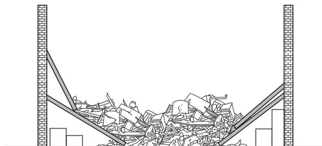
**FIGURE I.2(j) Fire Burn-Out Collapse Pattern — Roof/Floor Burn-Out — Heavy Wall Construction — URM or Tilt-Up.**
