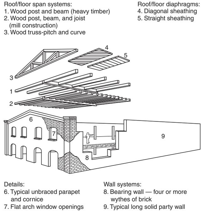
**FIGURE C.1(l) Unreinforced Masonry Bearing Wall, Example 1 of 3.**
