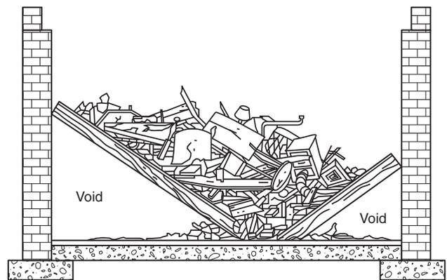
**FIGURE I.1(b) V-Shape Floor Collapse.** (Courtesy of U.S. Department of Civil Defense)
