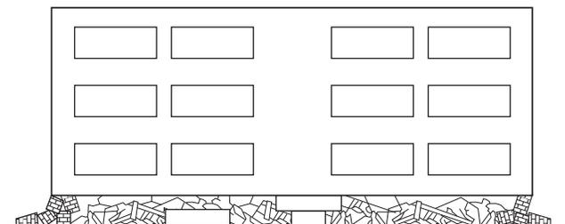
**FIGURE I.2(f) Soft First Story Collapse Pattern — Heavy Floor Construction.**
