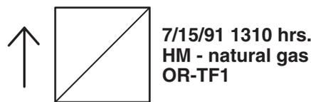
**FIGURE F.3(b) Structure Hazards Evaluation Markings.**
