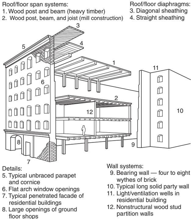
**FIGURE C.1(n) Unreinforced Masonry Bearing Wall, Example 3 of 3.**
