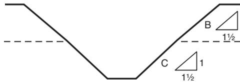
FIGURE B.1.4.1(f) B over C. [Source: 29 CFR 1926, Subpart P, Appendix B, Figure B-1.4.1(f)]
