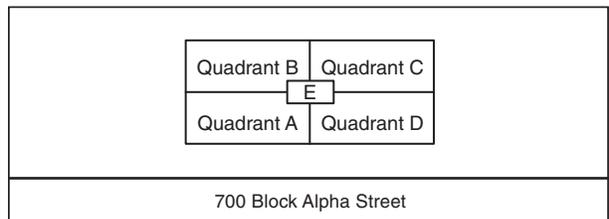
FIGURE F.2(c) Structure Identification Marking System Within a Geographic Area — Quadrants of a Single Structure.
