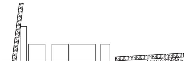
**FIGURE I.2(h) Wind Lift Collapse Pattern — Roof Off, Walls Collapse.**
