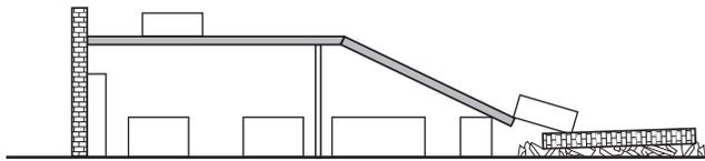
**FIGURE I.2(c) Wall-Fall Collapse Pattern — Heavy Wall — Tilt-Up Construction.**
