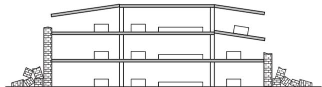
**FIGURE I.2(b) Wall-Fall Collapse Pattern — Heavy Wall — URM Construction.**
