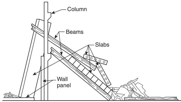
**FIGURE I.2(g) Random Fall Collapse Pattern — Precast Concrete Construction.**
