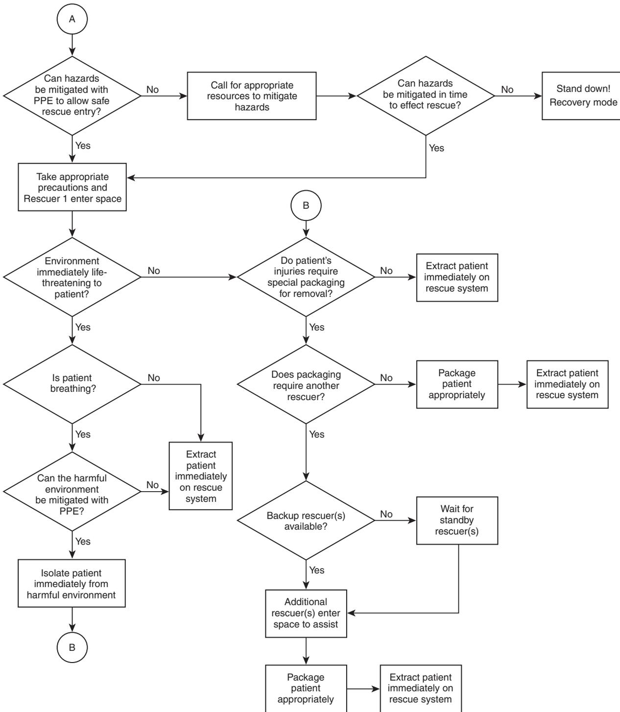
FIGURE G.1(c) Confined Space Rescue Pre-Incident Planning Form Flowchart. (Courtesy of Wright Rescue Solutions, Inc., 2001.)
