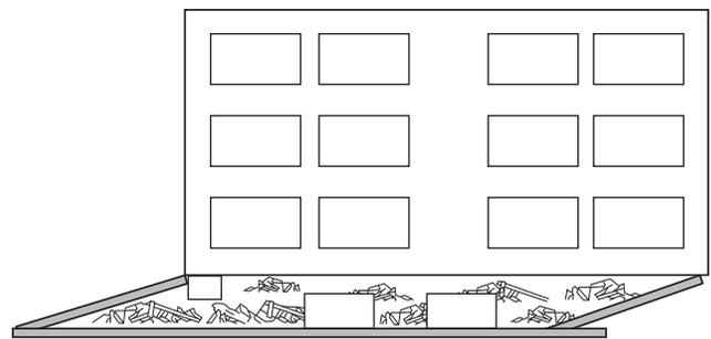
**FIGURE I.2(a) Offset Collapse Pattern — Light Frame Construction.**
