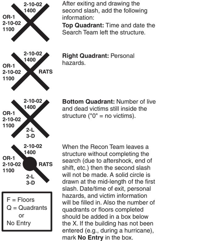
FIGURE F.4(b) Example of Structural Evaluation Markings.
