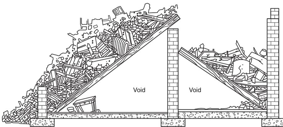
FIGURE I.1(e) A-Frame Floor Collapse. (Courtesy of U.S. Department of Civil Defense)
