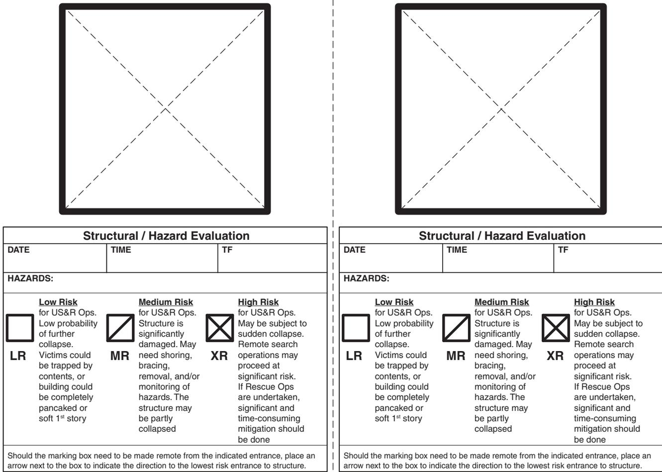
FIGURE F.3.1 Structure/Hazards Placard.
