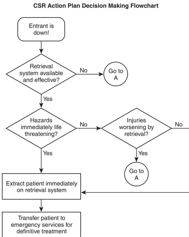
**FIGURE G.1(b) Confined Space Rescue Plan Decision Making Flowchart.** (Courtesy of Wright Rescue Solutions, Inc., 2001.)
