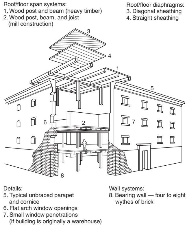
**FIGURE C.1(m) Unreinforced Masonry Bearing Wall, Example 2 of 3.**
