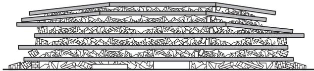
**FIGURE I.2(d) Pancake Collapse Pattern — Heavy Floor Construction.**
