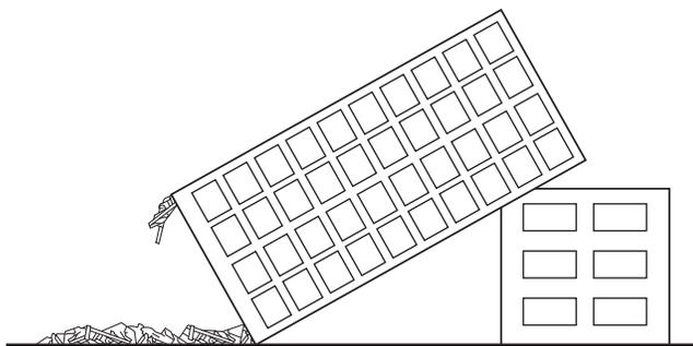
**FIGURE I.2(e) Overturn Collapse Pattern — Heavy Floor or Heavy Steel Construction.**
